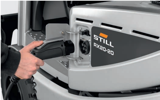
Optional onboard charger for decentralized charging without battery change
