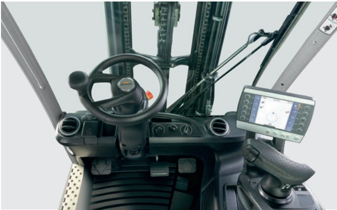
Workspace with display and control units, Joystick 4Plus and heating
