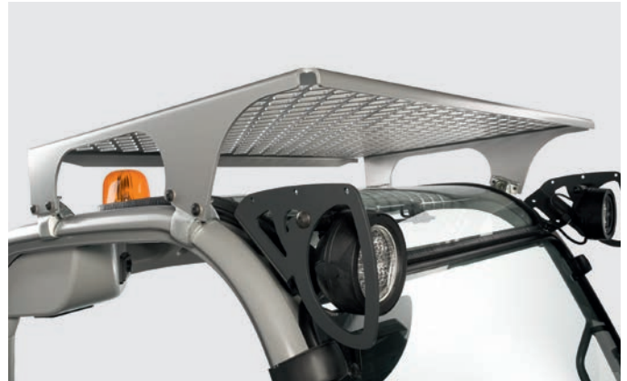
Additional protective grille roof
