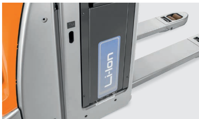
Increased operational hours thanks to fast interim charging with optional STILL Li-ion technology
