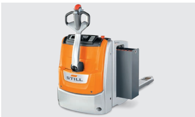
The EXH 25-30 is always available with lithium-ion technology and battery capacities of up to 500 Ah
