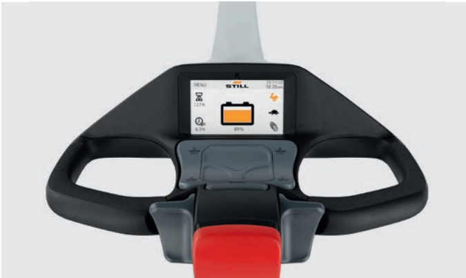
A quick glance at the optional touch display of the EXH 16-20 is all it takes to have all the relevant vehicle information clearly in front of you
