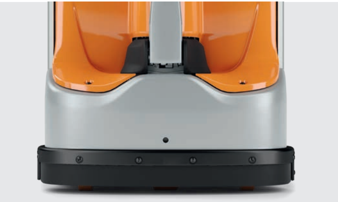
Safety guaranteed: the active foot stop on the EXH 16-20 stops and reverses the vehicle automatically on foot contact
