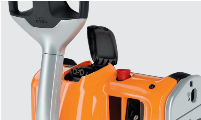
The optional quick-charging access for lithium-ion batteries on the EXH 16-20 makes charging processes even easier and faster
